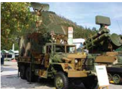
Low-Altitude Surveillance Radar http://www.lignex1.com:8001/en_US/product/product_detail.jsp?pid=19&scode1=&scode2=&scode3=&skey
