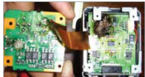
Types of damage caused by induced lightning strikes: electronic equipment, etc.
