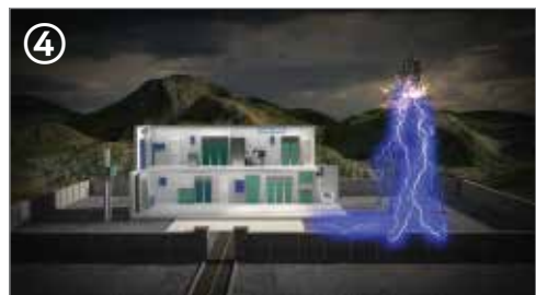
Flow into the lightning surge facility by the potential difference (induced lightning)
