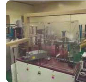
Lightning Current Rating test by KERI. Apply Class I (10x350 \mu s), 20kA surge current
