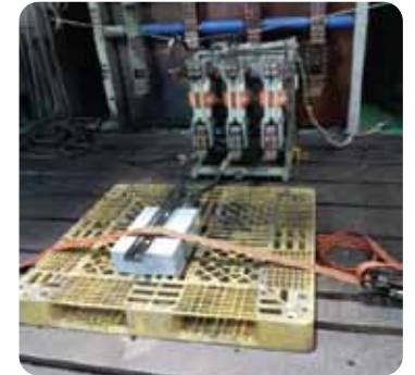
AC Fault Current Rating Test by KERI. Apply 60Hz, 30cycle, 3.7kA current
