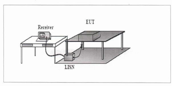
The continuous disturbance voltage on the AC mains in the frequency range from 0.15MHz to 30MHz was measured in accordance with IEC 61000-6-3. The mains terminal disturbance voltage was measured with the equipment under test(EUT) in the shielded room.
