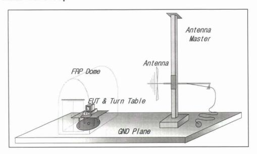
In the frequency range 30MHz to 1000MHz the radiated emission was measured in accordance with IEC 61000-6-3.
